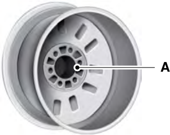
A Hub pilot bore.
