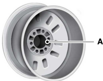
A Hub pilot bore.
