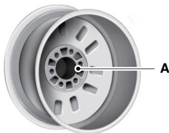
A Hub pilot bore.
