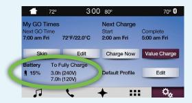
Check Battery status and estimated charge times using different voltage options.
