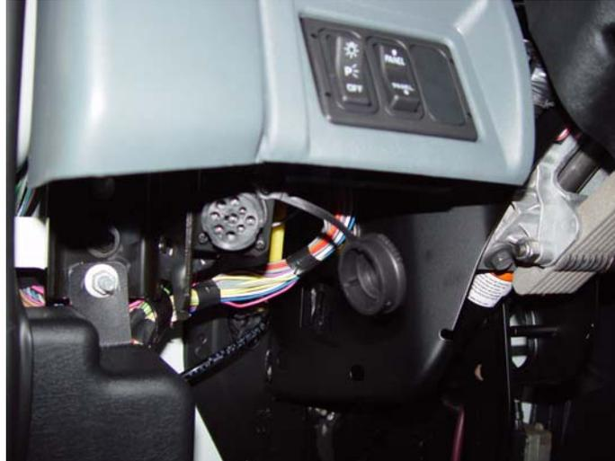
The other end of this 9-pin adapter cable connects to the Rotunda IC4COM serial cable. The serial interface cable then connects to the serial port on the IDS. Once the connections are made, the LEDs on the cable interface box should begin to scroll continuously across the various communications protocols (ATA, J1939, HS CAN etc).
