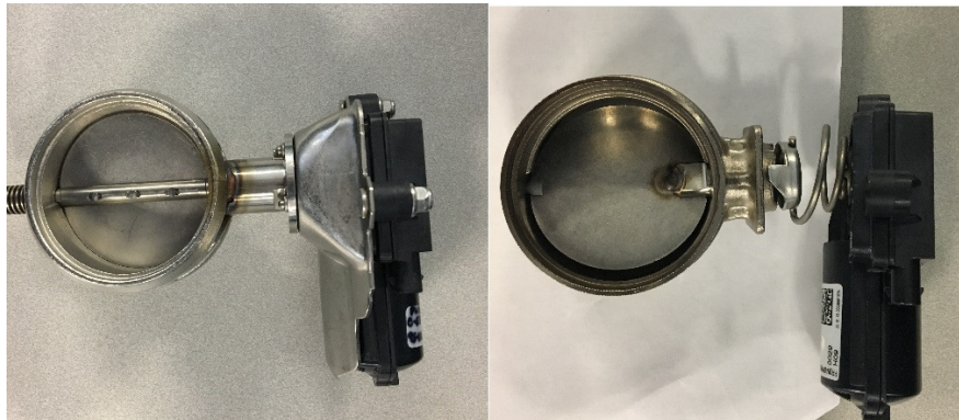
Fig. 1: Exhaust flow control valve with shield(left) and without shield (right: showing spring link)
