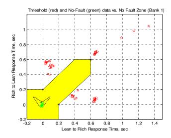
Example shown with lean-to-rich (0.2 sec), rich-to-lean (0.2 sec), and symmetric (0.6 sec) thresholds creating the yellow no-fault zone. The completeted monitor results in two measurements, a lean-to-rich response time and a rich-to-lean response time. These response time values are used as x-y pairs to make a single point and then compared to the no-fault zone. Anywhere in the yellow is a pass and outside the yellow is a failure.
