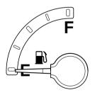
vehicle from empty indication, the amount of fuel that can be added will be less than the advertised capacity due to the reserve fuel.
