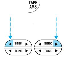
To set the minute, press and hold the CLK control and press the TUNE control:
