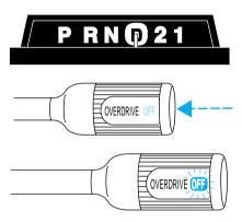
**Drive** – Not shown on the display. Activate by pressing the transmission control switch (TCS) on the end of the gearshift lever with the gearshift in the position. The TCIL (the word OFF) will illuminate on the gearshift lever. Transmission operates in gears one through three. Drive) provides more engine braking than (Overdrive) and is useful when:
