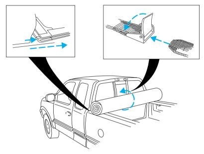
4. Starting from the opposite side of the vehicle, pull cover away from the side rail and roll the cover from rear to front.
