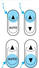
• Press the bottom portion of the rocker switch to open.
