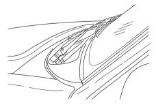
• Do not place objects over the defroster outlets. These objects can block airflow and reduce your ability to see through your windshield. Avoid placing small objects on top of the instrument panel. These objects may fall down into the defroster outlets and block airflow, in addition to damaging the climate control system.
