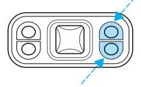
Press the control to move the seat forward, backward, up or down.
