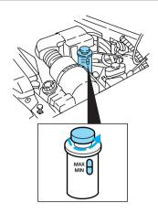
5. If the fluid is low, add fluid in small amounts, continuously checking the level until it reaches the range between the MIN and MAX lines. Be sure to put the cap back on the reservoir.
