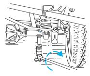
To lessen the risk of personal injury, do not put any part of your body under the vehicle while changing a tire. Do not start the engine when your vehicle is on the jack. The jack is only meant for changing the tire.
