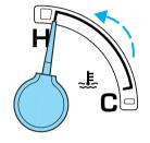
If the engine reaches a preset over-temperature condition, the engine will automatically switch to alternating cylinder operation. Each disabled cylinder acts as an air pump and cools the engine.
