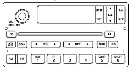
Your audio system is equipped with selective lighting, a unique lighting strategy. This lighting feature is operable when the headlamps are illuminated. During the operation of any selected mode, lighting for the individual function controls will either illuminate or turn off. Those controls which have a function for the specific mode of operation selected will be lit, while the controls which have no function for that mode will be turned off.
