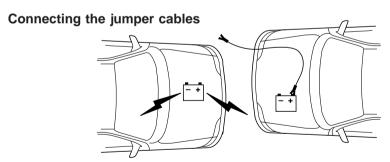
1. Connect the positive (+) booster cable to the positive (+) terminal of the discharged battery.
