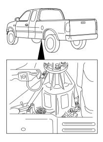
3. Add only enough fluid through the filler opening so that the fluid level is at the bottom of the opening.
