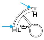
Add oil if needed (refer to *Engine oil* in the *Maintenance and care* chapter). If the oil level is correct, have your vehicle checked at your dealership or by a qualified technician.
