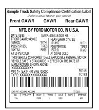
Exceeding the Safety Certification Label axle weight rating limits could result in substandard vehicle handling, performance, engine, transmission and/or structural damage, serious damage to the vehicle, loss of control and personal injury.
