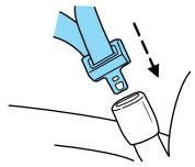
5. To put the retractor in the automatic locking mode, grasp the shoulder portion of the belt and pull downward until all of the belt is extracted and a click is heard.
