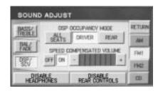
The recommended level for the speed compensated volume is from level 1 through level 3. When activated, level 1 is the minimum setting and level 7 is the maximum setting.
