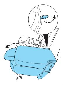
Always latch the vehicle seat to the floor, whether the seat is occupied or empty. If not latched, the seat may cause injury during a sudden stop.
