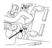
4. Make the final connection of the negative (-) cable to the exposed ground metal surface accessible on the side of the power steering pump reservoir bracket, facing the battery. **Do not** use fuel lines, engine rocker covers or the intake manifold as *grounding* points.
