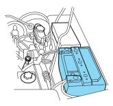
However, for severe usage or in high temperature climates, check the battery electrolyte level. Refer to the scheduled maintenance guide for the service interval schedules.
