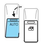
• Pull up (to the first detent) and hold the top portion of the switch to close.
