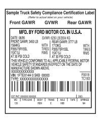
Exceeding the Safety Certification Label axle weight rating limits could result in substandard vehicle handling, performance, engine, transmission and/or structural damage, serious damage to the vehicle, loss of control and personal injury.
