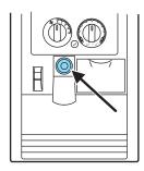
Another auxiliary power point is located on the right rear quarter panel. The power point is accessible from the liftgate.
