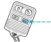
Pressing the power door UNLOCK control within the 20 second prearmed mode will return the vehicle to a disarmed state.
