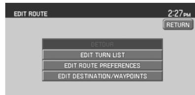
**DETOUR:** Press to select a portion of the route for the navigation system to avoid. Select the desired distance (between one and 100 miles) of the detour. A map for each alternative route will display on the screen. Select the desired route.
