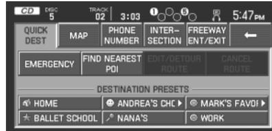
The system will allow you to input of a Freeway name, and an entrance or exit to that freeway. The entrance/exit list can be sorted alphabetically or by distance from the vehicle position. After selecting the desired intersection, the Destination Map will appear.
