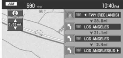
Regardless which guidance view is selected, a detailed intersection screen will appear on the right side of the map display when the vehicle is approaching the next turn.
