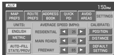
**AUTO-FILL STATE/PROV:** When selected, the State/Province field will be automatically filled in based on current location for destination entry. If it is not selected, the last State/Province will be displayed.
