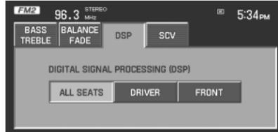
**SCV** (Speed Compensated Volume): Radio volume changes automatically with vehicle speed to compensate for road and wind noise. You may turn the feature on/off, and select a level of compensation between 1 and 7 by pressing the corresponding button.
