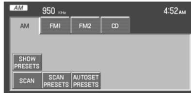
4. Press TUNE to adjust manually up (▲) or down (▼) the frequency band.
