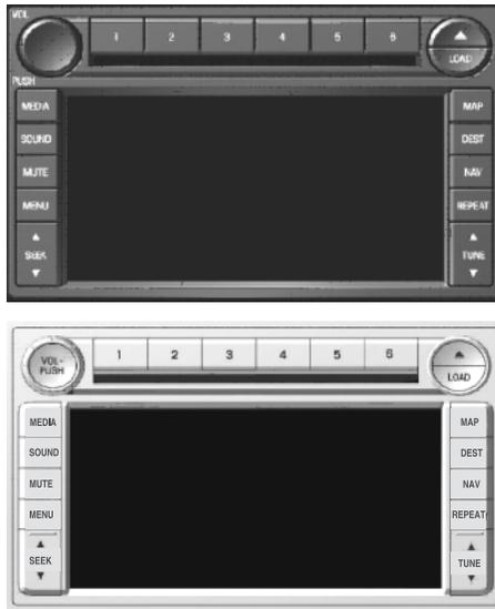
Your system has a large range of features, yet is easy to use. Guidance is shown on the display screen and is supplemented with voice prompts. The display screen provides full information for operating the system through the use of tabbed menus, text screens, and map displays. Screen selections are made by touching the desired selection on the touch screen.
