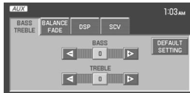
**BALANCE/FADE:** Press ◀ / ▶ to adjust the sound between the left and right speakers (Balance) and ▲ / ▼ to adjust the sound to the front and rear speakers (Fade).
