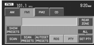
5. Press SHOW PRESETS to view the preset stations. To set or change a preset station, press and hold any of the presets while on the desired station. The new station will replace the previous one recorded.
