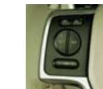
To return to a previously set speed faster than 30 mph, press RES. To disengage speed controls, depress the brake pedal or press OFF.
