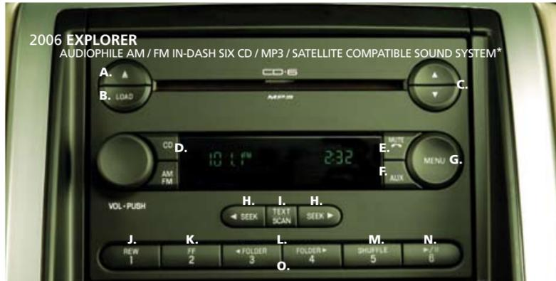
**A. CD Eject:** Press to eject a CD. Press and hold to auto eject all CDs present in the system. If there is no CD present, the display will read NO DISC.
