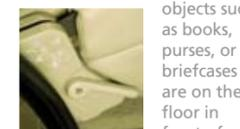
objects such as books, purses, or briefcases are on the floor in front of or under the seat. **1.** Lower the head restraints by pulling on the strap. **2.** Locate the handle on the side of the seat cushion by the door. **3.** Pull up on the handle and push the seatback forward toward the front of the vehicle.
