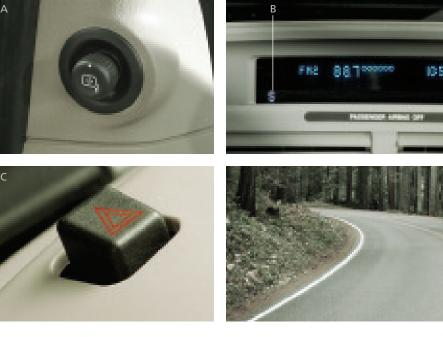
A. POWER SIDE VIEW MIRRORS – Rotate the control clockwise to adjust the right mirror, and counterclockwise to adjust the left mirror. Then move the control in the direction you wish to tilt the mirror. Return to the center position to lock the mirror in place.
