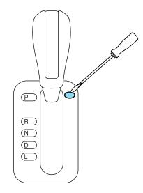
If it is necessary to use the above procedure to move the gearshift lever, it is possible that a fuse has blown or the vehicle's brakelamps are not operating properly. Refer to *Fuses and relays* in the *Roadside Emergencies* chapter.
