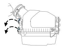
6. Replace the air filter housing cover and secure the clamps. Be sure that the air cleaner cover tabs are engaged into the slots of the air cleaner housing.
