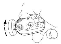
Likewise, when rotating the IKT to the 1 (LOCK) position in the ignition lock cylinder, the bottom edge of the IKT adjacent to the control can be utilized.
