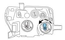
Handle a halogen headlamp bulb carefully and keep out of children's reach. Grasp the bulb only by its plastic base and do not touch the glass. The oil from your hand could cause the bulb to break the next time the headlamps are operated.
