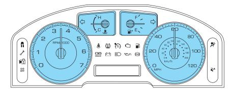
**Speedometer:** Indicates the current vehicle speed.
