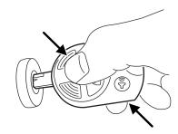
To gain more leverage when rotating the IKT in the ignition lock cylinder, you can readjust the location of your thumb to grasp the IKT on the outer edge next to the a control.
