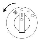
The autolamp system also keeps the lights on for a predetermined amount of time after the ignition switch is turned to LOCK. You can change the amount of time the lamps stay on by using the programming procedure that follows:
