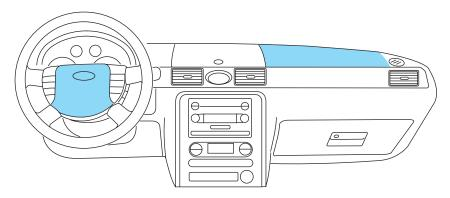
The airbag supplemental restraint system (SRS) is designed to work in conjunction with the safety belts to help protect the driver and front
