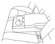
If your vehicle is equipped with cup holders and a storage compartment, they are located in the rear seat armrest. To access the cup holders, rotate armrest into use position. To open the storage compartment (if equipped), pull up on the latch.
