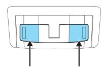
Your vehicle may also have reading lamps within the rear dome lamp(s). Press the switches on either side of the dome lamp to turn on the lamps.
