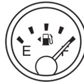
The arrow next to the fuel pump icon indicates which side of the vehicle the fuel filler inlet is located.
