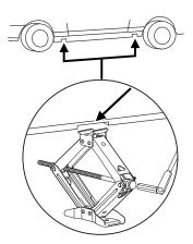
6. Lower the wheel by turning the jack handle counterclockwise.
