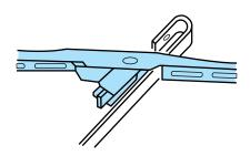
2. Attach the new wiper to the wiper arm and press it into place until a click is heard.
