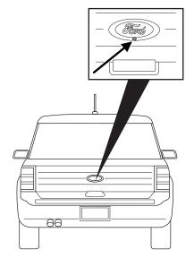
To use the camera system, place the transmission in R (Reverse); an image will display on the navigation screen. The area displayed on the screen may vary according to the vehicle orientation and/or road condition.
