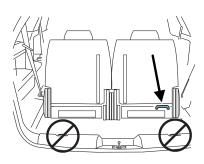
3. Clip the tether strap to the anchor as shown.
