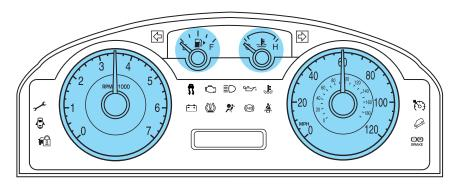
**Speedometer:** Indicates the current vehicle speed.
