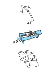
If you are stowing the flat tire, remove the L-shaped bolt from from the external pocket of the felt bag. With the 3rd row seat in the raised position, stand the flat tire in the rear of the vehicle with the tire's valve stem facing the rear of the
