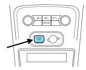
The 110V AC power point is located on the back of the center console.
