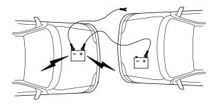
$2.\ \mbox{Remove}$  the jumper cable on the negative (-) connection of the booster vehicle's battery.
