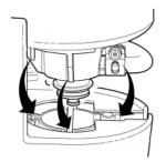
2. Once aligned, seat the sealant canister by lightly pushing down until you hear an audible click.
