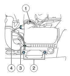
C. Remove the bolt cover (if equipped).
