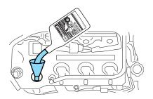
• Do not overfill the engine with oil. Oil levels above this mark may cause engine damage. If the engine is overfilled, some oil must be removed from the engine by an authorized dealer.
