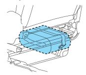
To replace the temporary mobility kit, open the Velcro® strap on the bag and slide the bag back under the driver's seat. Wrap the strap over the rear frame bar, loop it through the buckle and secure the bag to the seat frame.
