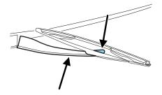
3. Grip tightly and press on the arm/blade joint from beneath and separate the blade from the arm.
