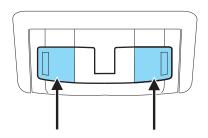
Your vehicle may have reading lamps within the rear dome lamp(s). Press the switches on either side of the dome lamp to turn on the lamps.
