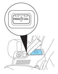
When the vehicle is turned off, the refrigerator/freezer will also turn off and will turn back on to the last used mode (freeze or cool) once the vehicle is restarted.
