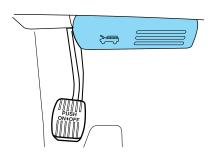
2. Go to the front of the vehicle and release the auxiliary latch that is located under the front center of the hood.
