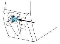
**Note:** The 110V AC power point is equipped with a safety cap and a safety twist tab. They both provide protection from inserting any object into the power point other than the 110V AC electrical device plug. The safety cap should always be in a closed position whenever the power point outlet is not in use.
