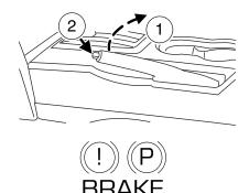
The BRAKE warning lamp will illuminate and will remain illuminated until the parking brake is released.
