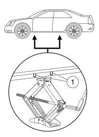
**WARNING:** To lessen the risk of personal injury, do not put any part of your body under the vehicle while changing a tire. Do not start the engine when your vehicle is on the jack. The jack is only meant for changing the tire.
