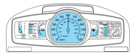
Displays unique hybrid vehicle gauges, along with many of the familiar gauges from a conventional gasoline vehicle.
