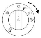
The autolamp system also keeps the lights on for a predetermined amount of time after the ignition switch is turned to off. You can change the amount of time the lamps stay on by using the programming procedure that follows:
