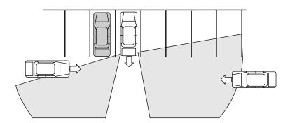
CTA coverage also decreases when parking at shallow angles (refer to figure for approximate zone coverage areas [sensor obstructed to vehicle on left]).
