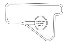
levels in both reservoirs need to be maintained. When the engine is cold, check the level of M/E coolant in the reservoir. The coolant should be at the FULL COLD level as shown on the side of the coolant reservoir.
