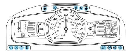
Warning lights and gauges can alert you to a vehicle condition that may become serious enough to cause extensive repairs. A warning light may illuminate when a problem exists with one of your vehicle's functions. Many lights will illuminate when you start your vehicle to make sure the bulbs work. If any light remains on after starting the vehicle, refer to the respective system light explanation later in this section for additional information.
