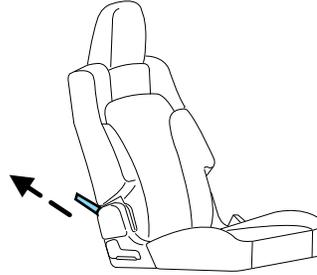
3. To return the seatback to the floor from tumbled position, rotate the seat down until you hear it latching to the floor.
