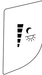
The lights come on whenever the ignition is in either on or in the accessory position and the parking lamps or headlamps are on.
