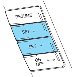
The ACC may apply the brakes to slow the vehicle down to the new set speed. The set speed will display continuously in the message center while ACC is active.
