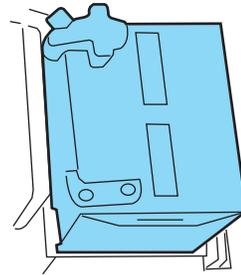
**If your battery has a cover/shield, make sure it is reinstalled after the battery has been cleaned or replaced.**
