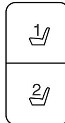
A position can only be recalled when the transmission gearshift is in Park (automatic transmission). A memory seat position may be programmed at any time.
