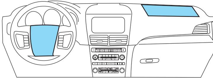
The airbag supplemental restraint system (SRS) is designed to work in conjunction with the safety belts to help protect the driver and front outboard passenger from certain upper body injuries. The term “supplemental restraint” means the airbags are intended as a supplement to the safety belts. Airbags offer the most protection when used with safety belts for crash conditions for which airbags are designed to deploy. Airbags do not offer any protection in crashes for which they do not deploy.
