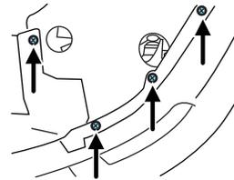
After removing to allow free access to the front fog lamp bulb and electrical wire harness, the splash shield flap should be able to be repositioned.
