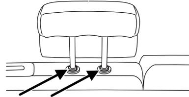
Properly adjust the head restraint so that the top of the head restraint is even with the top of your head and positioned as close as possible to the back of your head. For occupants of extremely tall stature, adjust the head restraint to its full up position.
