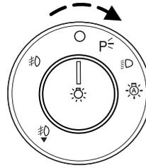
The autolamp system also keeps the lights on for a predetermined amount of time after the ignition switch is turned to off. You can change the amount of time the lamps stay on by using the programming procedure that follows:
