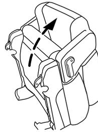
3. To return the seatback to the floor from tumbled position, rotate the seat down until you hear it latching to the floor.
