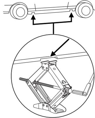
6. Lower the wheel by turning the jack handle counterclockwise.
