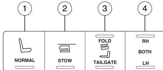
Press the seat selection button (4) to select either right-hand seat, the left-hand seat or both. First select the seat you would like to adjust, then select one of the following:
