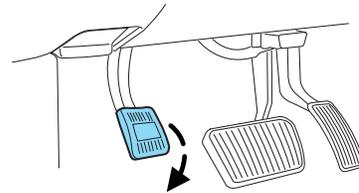
**Note:** If the vehicle is driven with the parking brake applied, a chime will sound.
