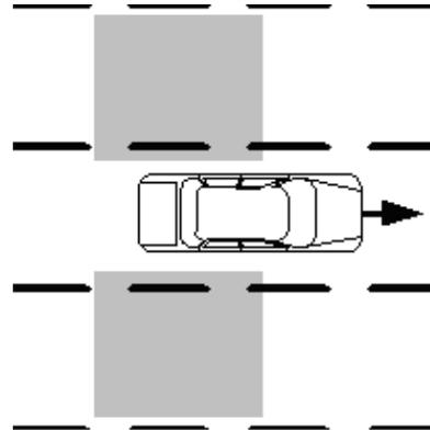
**⚠ WARNING:** To help avoid injuries, NEVER use the BLIS® as a replacement for using the side and rear view mirrors and looking over your shoulder before changing lanes. BLIS® is not a replacement for careful driving and only an assist.
