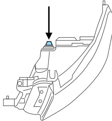
HORIZONTAL AIM IS NOT REQUIRED FOR THIS VEHICLE AND IS NON-ADJUSTABLE.
