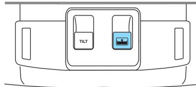
To open the panoramic Vista Roof™ press and release the
