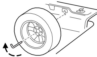
clockwise into the threaded hole in the vehicle until the tire is secured.
