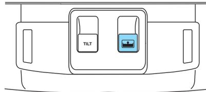
To open the panoramic Vista Roof™ press and release the
