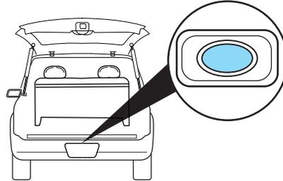
**Note:** For the best performance allow the power system to open the liftgate after pressing the control. Manually pushing or pulling the liftgate may activate the system's obstacle detection feature and stop the power operation.
