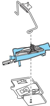
**If you are stowing the flat tire,** remove the L-shaped bolt from the external pocket of the felt bag. With the 3rd row seat in the raised position, stand the flat tire in the rear of the vehicle with the tire's valve stem facing the rear of the vehicle. Fasten the flat tire to the vehicle by inserting the L-shaped bolt through one of the lug bolt holes in the wheel and turning
