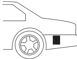
**Note:** The BLIS® typically will not detect parked vehicles, humans, animals, or infrastructure (fences, guard rails, trees, etc.). The BLIS® does not function when the transmission is in R (Reverse) or P (Park). The BLIS® does not provide any additional warning when your turn signal is activated.
