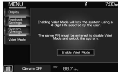
3. Enter a four digit Personal Identification Number (PIN) and press 'Enter'. The system will ask you to re-enter the PIN. Once entered, select 'Enable' to activate Valet mode. The system is then locked until the correct four digit PIN is entered.
