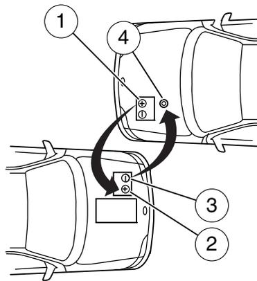
**Note:** Do not attach the negative (-) cable to fuel lines, engine rocker covers, the intake manifold or electrical components as grounding points.
