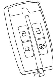
The IA key also contains a removable mechanical key blade that can be used to unlock the driver door. To release the mechanical key blade, press the release button on the back of the transmitter and slide the blade out.
