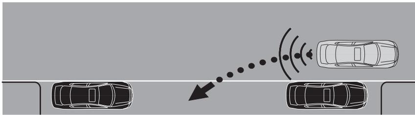
When you determine the vehicle is back far enough or you hear a solid tone from the reverse sensing system, bring the vehicle to a complete stop and move the gearshift to D (Drive). The message center will now display **PULL FORWARD USE CAUTION** followed by a chime.
