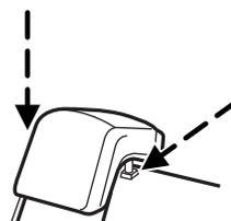
Properly adjust the head restraint so that the top of the head restraint is even with the top of your head and positioned as close as possible to the back of your head. For occupants of extremely tall stature, adjust the head restraint to its full up position.
