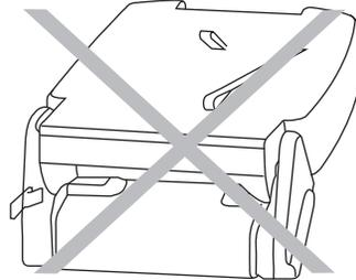
**Note:** In order to allow the seat to latch in the stowed position, do not stow objects under the seat before stowing.
