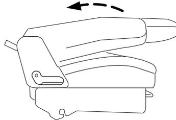
**Note:** The seatback will not raise if the rear latch hooks are not properly engaged to the floor striker. If the seatback does not raise, then repeat Steps 3 and 4.
