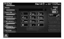
4. Scroll using  $\blacktriangle$  /  $\blacktriangledown$  on the touchscreen to cycle through a list of 15 predefined text messages you can send from SYNC<sup>®</sup>.
