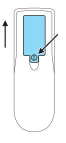
Remove the screw and unlatch the battery cover to access the batteries. The remote control unit uses two AAA batteries which are supplied with the unit.
