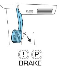
The BRAKE warning lamp in the instrument cluster illuminates and remains illuminated (when the ignition is turned on) until the parking brake is released.
