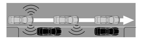
When the system has found a space, the message center will display SPACE FOUND PULL FORWARD followed by a chime. Drive forward until the message center displays SPACE FOUND STOP followed by a chime. When you stop the vehicle in position to begin parking, the message center displays REMOVE HANDS PUT IN REVERSE. The driver should always come to a complete stop before changing gears. 276
