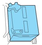
If you see any corrosion on the battery or terminals, remove the cables from the terminals and clean with a wire brush. You can neutralize the acid with a solution of baking soda and water.
