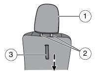
To fold the head restraint, pull the fold strap. To place the head restraint back to the upright position, pull up on the head restraint.
