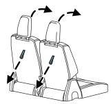
**WARNING:** To minimize the risk of neck injury in the event of a crash, passenger occupants should not sit in the vehicle until the head restraint is placed in its proper position.
