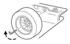
clockwise into the threaded hole in the vehicle until the tire is secured.
