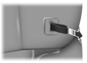
4. Pull the strap located on the back of the seat to fold the front passenger seatback.
