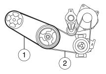
1. Short drivebelt is on first pulley groove closest to engine (not applicable to vehicles with electric power assisted steering).
