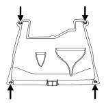
Some vehicles may be equipped with an aero-shield under the engine. This shield needs to be removed for service, including oil and filter changes. It is secured with four quick release fasteners.
