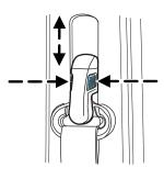
**WARNING:** Position the safety belt height adjusters so that the belt rests across the middle of your shoulder. Failure to adjust the safety belt properly could reduce the effectiveness of the safety belt and increase the risk of injury in a collision.
