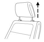
2. Simultaneously press and hold both the adjust/release button and the unlock/remove button, then pull up on the head restraint.
