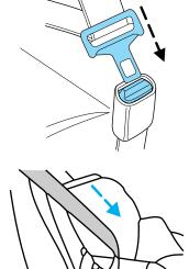
5. To put the retractor in the automatic locking mode, grasp the shoulder portion of the belt and pull downward until all of the belt is pulled out.
