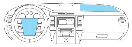
The airbag supplemental restraint system (SRS) is designed to work in conjunction with the safety belts to help protect the driver and front outboard passenger from certain upper body injuries. The term "supplemental restraint" means the airbags are intended as a supplement to the safety belts. Airbags offer the most protection when used with safety belts for crash conditions for which airbags are designed to deploy. Airbags do not offer any protection in crashes for which they do not deploy.
