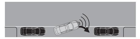
When you determine the vehicle is far enough forward or a solid tone from the forward sensing system (if equipped) is heard, bring the vehicle to a complete stop and move the gearshift to R (Reverse). The message center may display BACK UP SLOWLY USE CAUTION followed by a chime. The system may offer subsequent backward and forward maneuvers before proceeding to the finish phase.
