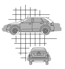
As a result of the above dimensional differences, crossover vehicles often will have a higher center of gravity and a greater difference in center of gravity between the loaded and unloaded condition.
