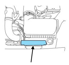
D. Remove two bolts that attach the air filter assembly to the front of the vehicle (2).
