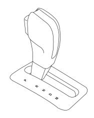
**WARNING:** Always set the parking brake fully and make sure the gearshift is latched in P (Park). Switch the ignition off and remove the key whenever you leave your vehicle.
