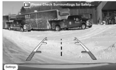
When the rear camera delay function is ON, it extends the display of the camera image into Drive mode until vehicle speed is greater than 5 mph (8 km/h). This is useful when trying to engage/disengage a trailer. Once you shift out of R (Reverse), the image will be removed from the screen. The default for the rear camera delay is off.
