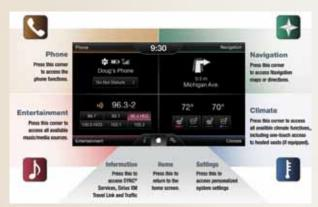
Use the four corner, four color touch screen to explore and interact with your vehicle. The touch screen works the same way traditional controls, knobs and buttons do. Simply press the various corners on your touch screen to personalize the many features and settings of your vehicle all in one place. The system provides easy interaction with your cellular phone, multimedia entertainment, climate controls and navigation system.\*
