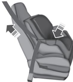
8. Remove remaining slack from the belt. Force the seat down with extra weight, e.g., by pressing down or kneeling on the child restraint while pulling up on the shoulder belt in order to force slack from the belt.
