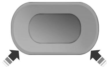
The control is located on the outboard side of the seat. Press the forward or rearward side of the control for more or less support.
