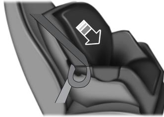
5. To put the retractor in the automatic locking mode, grasp the shoulder portion of the belt and pull downward until all of the belt is pulled out.
