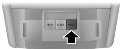
Press and hold the **VENT** control to open the windows.
