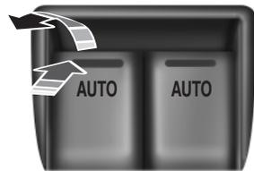
Press the switch to open the window.
