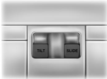
Press and release the **SLIDE** control to open the moonroof. The moonroof will stop short of the fully opened position.
