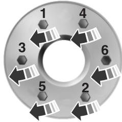
17. Remove the jack and fully tighten the lug nuts in the order shown and reinstall the wheel cover. See *Wheel Lug Nut Torque Specifications* later in this chapter for the proper lug nut torque specification.
