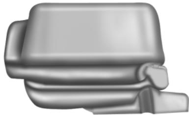
2. With the latch released the seatback can be lowered into the load floor position.
