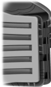
8. Replace the air filter housing cover and secure the clamps. Be careful not to crimp the filter element edges between the air filter housing and cover and ensure that the tabs on the edge are properly aligned into the slots.
