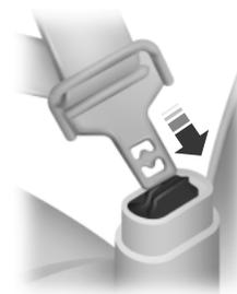
4. Insert the belt tongue into the proper buckle (the buckle closest to the direction the tongue is coming from) for that seating position until you hear a snap and feel the latch engage. Make sure the tongue is latched securely by pulling on it.
