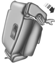
1. Push the seat down and latch to the floor.
