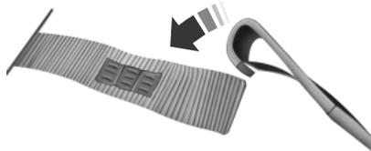
3. Clip the tether strap through the anchor loop as shown. If the tether strap is clipped incorrectly, the child safety seat may not be retained properly in the event of a collision.
