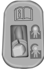
The childproof locks are located on the rear edge of each rear door and must be set separately for each door.
