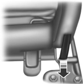
1. Pull the strap located at the bottom outboard of the seat back to release the seat from the floor, and rotate the seat up towards the front seat.
