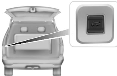
Press and release the control on the left rear quarter panel. A chime will beep once if conditions are not correct to start an operation (i.e., the vehicle is out of park). In a normal close, the chime will begin just before the gate starts to move and continue for a total of three seconds.
