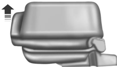
3. To return the seat to the upright position, lift the seatback until the latch is fully engaged.
