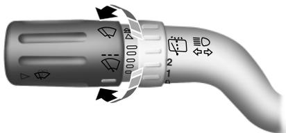
Use the rotary control to adjust the sensitivity to one of the interval moisture settings. The wipers will not cycle until moisture is detected on the windshield. The wiper speed will vary based on the amount of moisture detected on the windshield and the sensitivity setting. The
