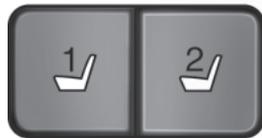
2. Press and hold memory button **1** (on the side of the driver's seat) for five seconds. A tone will sound after about two seconds. Continue to hold until a second tone is heard.
