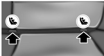
The locator symbols are on round plastic buttons for the center seat and on rectangular tags for the outboard seats.
