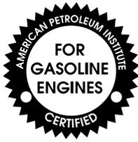
Only use oils certified for gasoline engines by the American Petroleum Institute (API). An oil with this trademark symbol conforms to the current engine and emission system protection standards and fuel economy requirements of the International Lubricants Specification Advisory Council (ILSAC), comprised of U.S. and Japanese automobile manufacturers.
