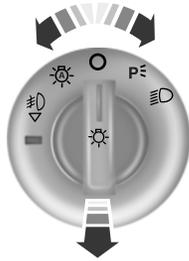
The control also operates the fog lamps. The fog lamps can be turned on when the control is in the parking lamps on, headlamps on, or autolamps positions and the high beams are not turned on.
