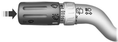
Press the end of the stalk to activate the washer.
