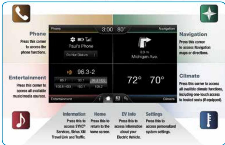
Use the four-corner, four-color touchscreen to explore and interact with your vehicle. The screen works the same way as traditional controls, knobs and buttons do. Press the various corners on your touchscreen to personalize the many features and settings of your vehicle. The system provides easy interaction with your cellular phone, multimedia entertainment, climate controls and navigation system\*.
