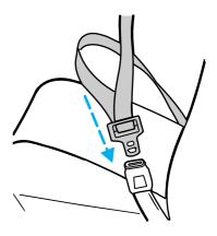
2. Grasp the shoulder belt portion and pull downward until the entire belt is extracted.
