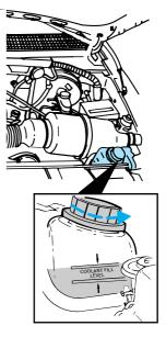
Check the coolant level in the coolant recovery reservoir the next few times you drive the vehicle. If necessary, add enough of a 50/50 mixture of coolant and water to bring the liquid level to the fill line on the reservoir.
