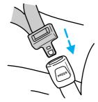
5. To put the retractor in the automatic locking mode, grasp the shoulder portion of the belt and
