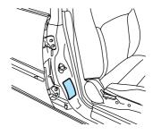
The cold pressure amount is listed on the Safety Compliance Certification Label located on the inside driver door latch pillar.
