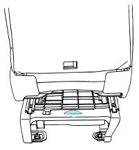
3. Route the child safety seat tether strap over the back of the front right-hand passenger seat as shown.
