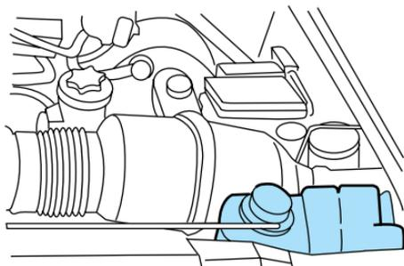
If the engine coolant has not been checked for a long period of time, the engine coolant reservoir may eventually empty. If this occurs, add engine coolant to the coolant reservoir. For more information on engine coolant maintenance, refer to *Adding engine coolant* in this chapter.
