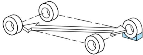
6. Loosen each wheel lug nuts one-half turn counterclockwise but do not remove them until the wheel is raised off the ground.
