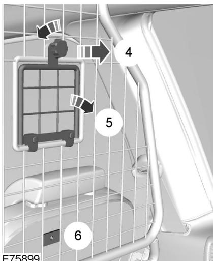
1. Loosen the handwheel and remove it **4**.
