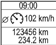
Press the **up** and **down** arrow buttons on the steering wheel to scroll through the trip computer displays. See **Trip Computer** (page 98).
