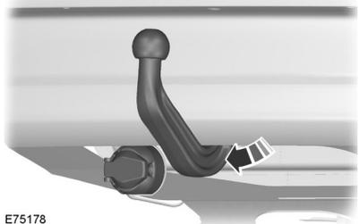
1. Insert the key into the handwheel and turn it clockwise to unlock.
