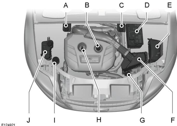
A Brake and clutch fluid reservoir (right-hand drive). See **Brake and Clutch Fluid Check** (page 245).
