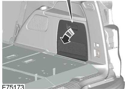
You can turn the retractable tow ball arm through 90 degrees using the handwheel **A**.
