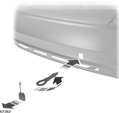
Insert your finger into the hole on the underside of the cover and prise off the cover. Install the towing eye.
