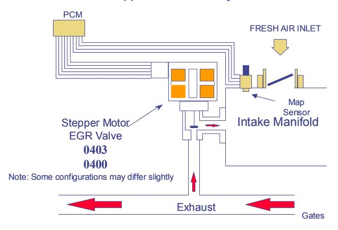
The Non-Intrusive Stepper Motor EGR Monitor consists of an electrical and functional test that checks the stepper motor and the EGR system for proper flow.
