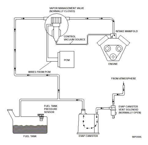
The evap system integrity test is done under two different sets of conditions - first a cruise test is performed to detect 0.040" dia leaks and screen for 0.020" leaks. If a 0.020" dia leak is suspected during the cruise test, an idle test is performed to verify the leak under more restrictive, but reliable, cold-start-idle conditions.
