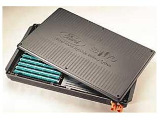
Nickel-metal hydride batteries (NiMH) have a much longer life cycle than lead acid batteries. In addition to electric vehicles and HEVs, they are often used in consumer electronics, computers and medical equipment.
