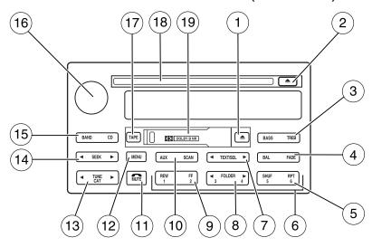
1. **EJ (Eject):** Press to stop and eject a tape.
