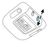
Press the  $\triangle$  portion of the VENT control to open the power rear quarter windows.
