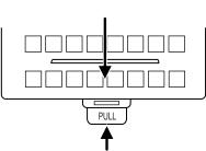
To reinstall the fuse box cover, place the top part of the cover on the fuse panel, then push the bottom part of the cover until you hear it click shut. Gently pull on the cover to make sure it is seated properly.
