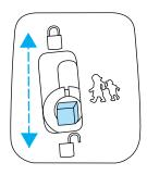
Move lock control up to engage the childproof lock. Move control down to disengage childproof locks.
