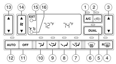
1. **A/C control:** Uses outside air to cool the vehicle. Press to turn on/off in all modes except www or \*\*.
