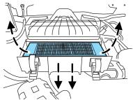
The air filter box needs to be free of any debris before installing a new air filter.
