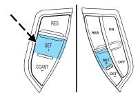
• Use the accelerator pedal to get to the desired speed. When the vehicle reaches that speed press and release the SET + control.
