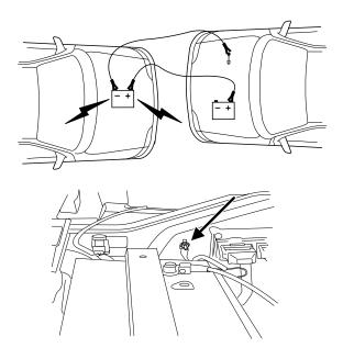
4. Make the final connection of the negative (-) cable to the jump starting stud located in the rear of the engine compartment, near the battery. **Do not** use fuel lines, engine rocker covers or the intake manifold as *grounding* points.
