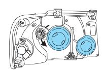
7. Once the bulb covers are removed, the bulbs can be removed by turning them counterclockwise and then pulling the bulbs straight out.
