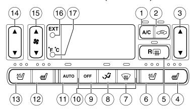
1. **A/C control:** Press to engage/disengage the air conditioning in all modes except defrost and floor/defrost. Uses outside air to cool the vehicle.
