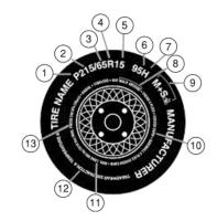
7. **H:** Indicates the tire's speed rating. The speed rating denotes the speed at which a tire is designed to be driven for extended periods of time under a standard condition of load and inflation pressure. The tires on your vehicle may operate at different conditions for load and inflation pressure. These speed ratings may need to be adjusted for the difference in conditions. The ratings range from 81 mph (130 km/h) to 186 mph (299 km/h). These ratings are listed in the following chart.
