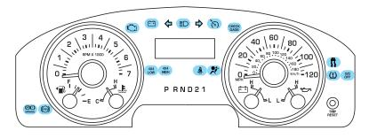
Warning lights and gauges can alert you to a vehicle condition that may become serious enough to cause expensive repairs. A warning light may illuminate when a problem exists with one of your vehicle's functions. Many lights will illuminate when you start your vehicle to make sure the bulb works. If any light remains on after starting the vehicle, have the respective system inspected immediately.
