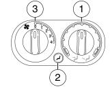
2. **Mode selector:** Press to select between air flow to 🗸 (Floor) or 🕻 (Panel).
