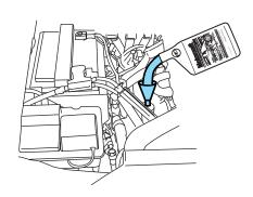
• Do not overfill the engine with oil. Oil levels above this mark may cause engine damage. If the engine is overfilled, some oil must be removed from the engine by a qualified service technician.
